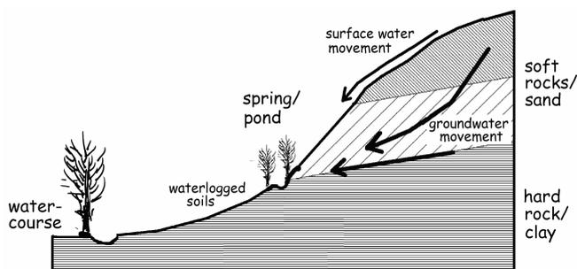
In some areas where the rocks are very porous (such as limestone or chalk) large streams emerge from the side of the hill. This allows you to take buckets of water with ease! The important thing about groundwater is that it's pretty much sterile (there are no 'bugs' in it) because it's been filtered through the soil and rocks. The principle hazard with
