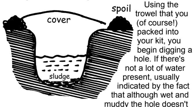
fill with water right away, dig a small narrow hole, just big enough to get a cup inside. If the ground is well saturated, and the hole fills as you dig, then a larger hole can be excavated to fit a saucepan into. Go down as far as you can easily go, say to the depth of your elbow. As you dig compact the excavated spoil around the hole in a ring. This will stop any contaminated surface water flowing into your hole if it rains.
