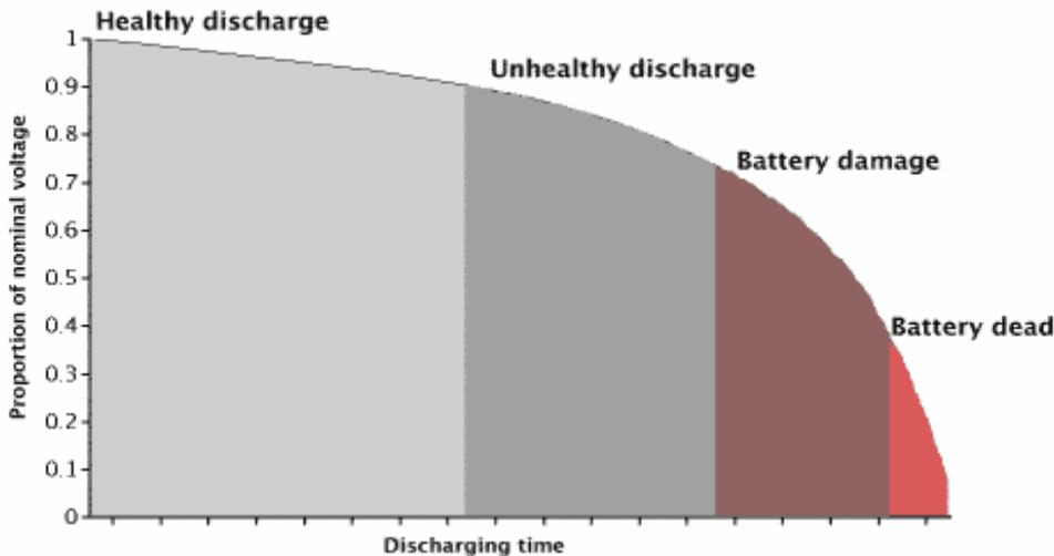
reduce the build-up of compounds that shorten the life of the battery. DC-SLAs will discharge down to about 10V without causing serious damage. But below that and the battery will begin to accumulate damage, shortening the life.
