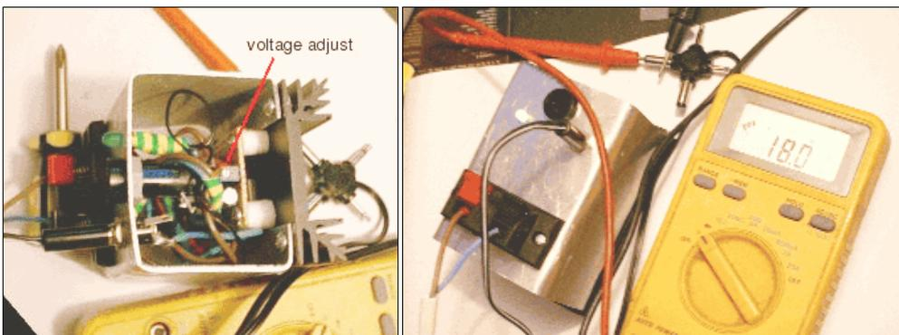
of the battery if done regularly). Therefore, with a 24 volt battery, you can produce any voltage between 8 volts and 19 volts.
