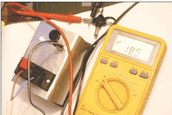
Converting from a fixed battery voltage down to a pre-set DC voltage is more efficient (around 95% – 98%). But to do this you need a regulator. The Tech2 Regulator is designed to produce DC voltages from 5V up to 32V, using different 'packs' of batteries producing a nominal voltage of 12V, 18V, 24V, 30V or 36V. This is more efficient because the regulator need only regulate the voltage between 3V to
