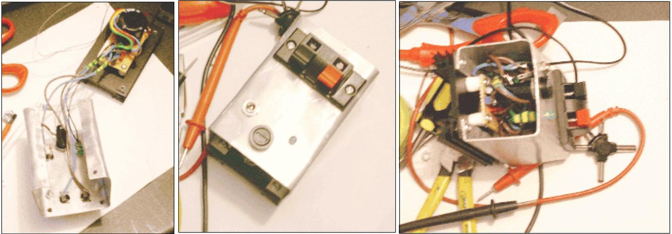
need to tidy up the wires inside. There is not a serious safety problem with the unit because at most it only uses 36 volts. But problems may arise if any wires connected to the positive of the battery supply touch the case – they'll arc or spark. For this reason you should tidy the wires up to ensure they don't loop outside of the case (if you use a proper box for the unit you won't have this problem).
