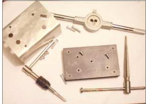
The front panel was drilled to mount the components. The holes were roughly drilled and then enlarged to the required size using a reamer.
