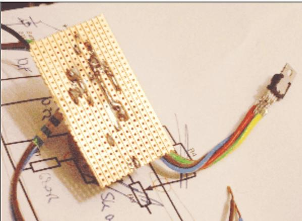
One significant consideration is the power capacity of stripboard. When operating at the regulator's limits the copper strips will be required to conduct up to 2.5 Amps at 40 volts. To ensure that the copper strips do not heat up, solder is 'mounded' along the copper strips between the components that carry the highest power load.
