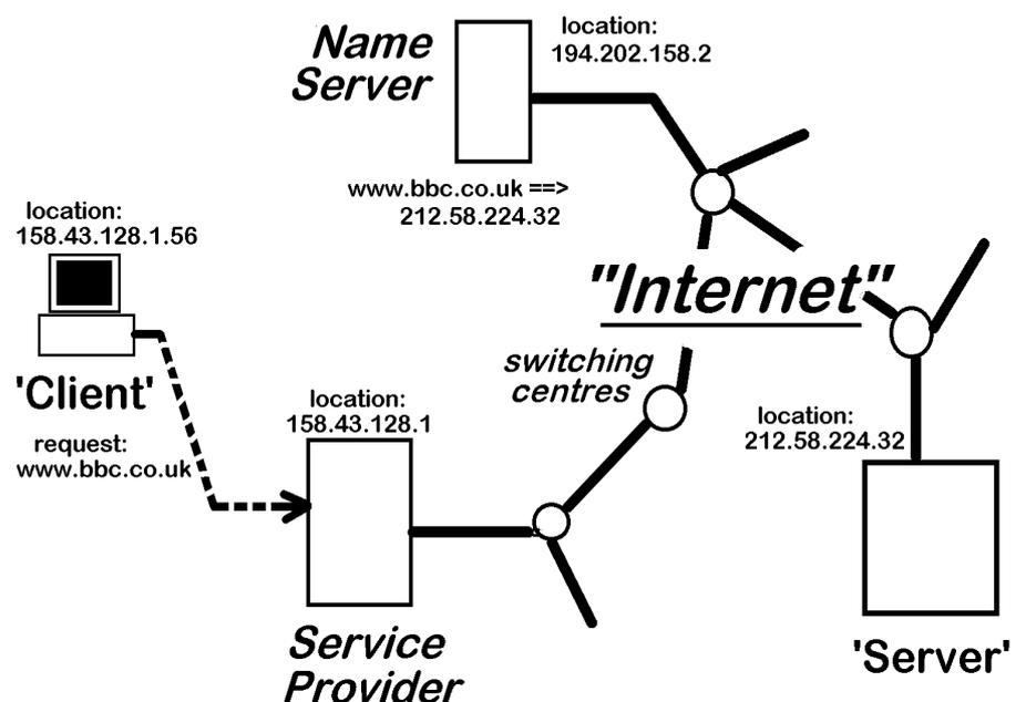
This URL must be translated into a numeric address. To do this, your computer (i.e. the *client*) first sends the URL address to a *name server*. The name server has its own pre-assigned numeric address (in our example, 194.202.158.2) to which your computer sends your request. The name server sends back to the client a numeric address that corresponds to the location of the server "www.bbc.co.uk", in this case 212.58.224.32.
