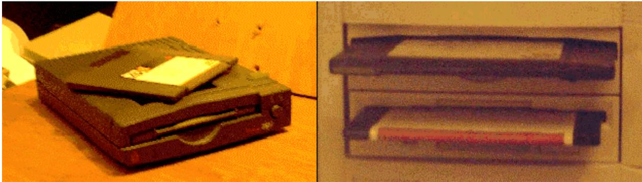
Left -an external ZIP drive. Right, top -an internal ZIP drive, with a floppy disk drive below for comparison
